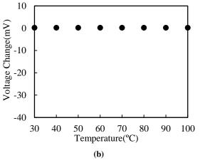
Fig.4 (a) Hydrogen response and (b) temperature dependence of the bridge-type sensor.
