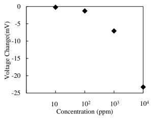
Fig.5 Hydrogen-dependent response characteristics of the sensor.
