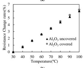
Fig.3 Effect of Al $_2O_3$  film. (a) The hydrogen response and (b) the temperature dependence of the Pt/TiN resistors.
